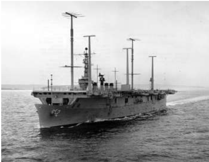
USS Wright (CC-2) under way on 17 June 1963, following her conversion to National Emergency Command Post Afloat. An extensive array of large communications antennas was installed on her flight deck to provide presidential command facilities. Naval History and Heritage Command photograph #NH 97621
