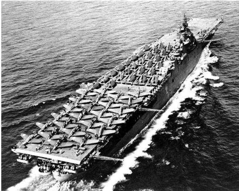
USS Essex (CV-9) underway in May 1943. The aircraft on her flight deck include 24 SBD scout bombers (located aft), about 11 F6F fighters (after midships area) and some 18 TBF/TBM torpedo planes (amidships). National Archives photograph #80-G-68097
