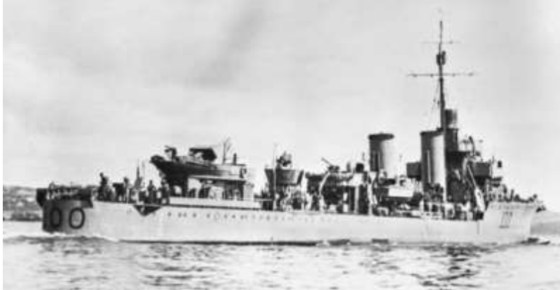
HMAS Stuart , of 1,530 tons displacement, was armed with five 4.7-inch guns and smaller anti-aircraft guns, six 21-inch torpedo tubes, and depth charges, and could make a top speed of 36 knots. Australian War Memorial 066092
