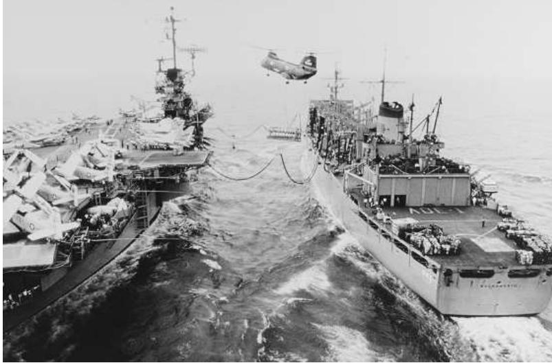
USS Sacramento (AOE-1) transfers fuel and ammunition through hoses and highlines to USS Hancock (CVA-19), while a CH-46 Sea Knight helicopter supports crated Mark 77 fire bombs (napalm) being transferred to the carrier, 9 August 1966. National Archives photograph #K-31344
