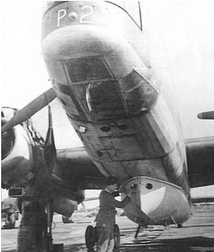
An airborne lifeboat fitted to a Warwick aircraft of the RAF Air-Sea Rescue service, England, circa November 1944.
