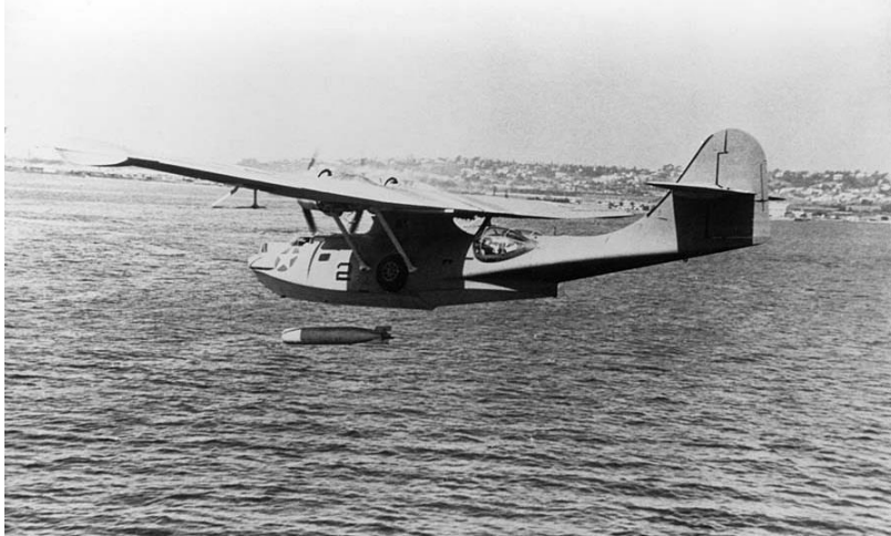
PBY-5A Catalina drops an aircraft torpedo during tests in 1942-1943. Patrol Wing Ten utilized the earlier model PBY-4 aircraft during the Defense of the Java Sea. U.S. Naval History and Heritage Command Photograph #NH 94118
